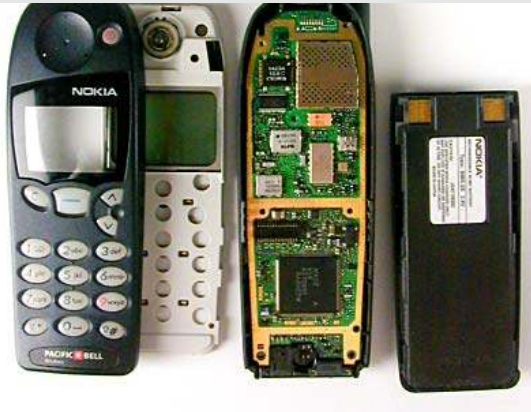
The parts of a cell phone
