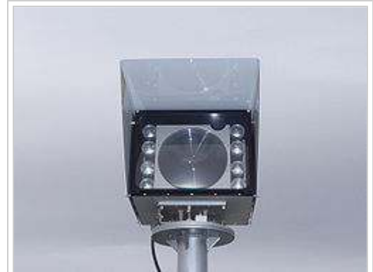
An 8-beam free space optics laser link, rated for 1 Gbit/s at a distance of approximately 2 km. The receptor is the large disc in the middle, the transmitters the smaller ones. To the top and right side a monocular for assisting the alignment of the two heads.
